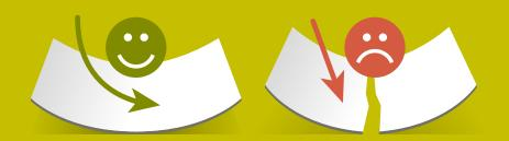
**HUMIDIFY** Moisten the panel to facilitate bending.
